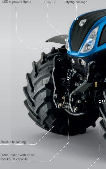
Front linkage with up to 3568kg lift capacity
